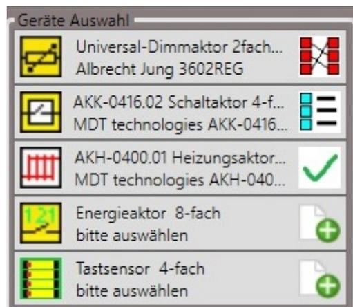
If you press a pattern device, first is the device selection from the ETS catalog.
